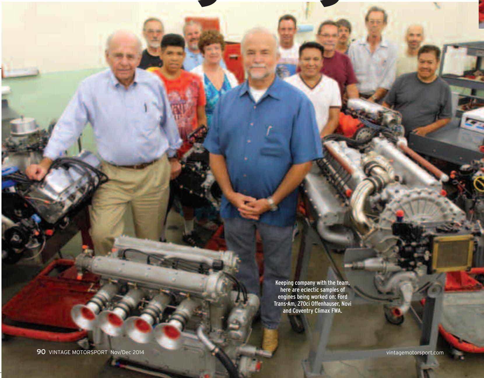
Keeping company with the team, here are eclectic samples of engines being worked on: Ford Trans-Am, 270ci Offenhauser, Novi and Coventry Climax FWA.
